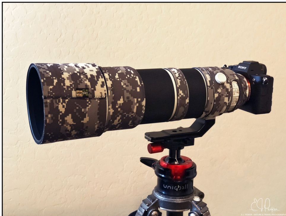
Sony a7R IV with 200-600mm lens, LensCoat, and Wimberley Foot mounted on a UniqBall gimbal style ballhead. (I am not using the LensCoat cover over the zoom and focus rings)
